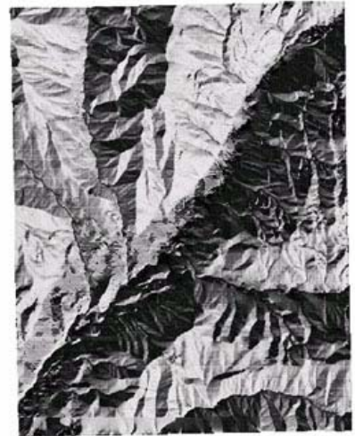
Hill shading on Aspen elevation data
